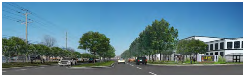
Figure 77 Oblique drawing of narrow median concept applied to Kings Highway at Gills Neck Road
